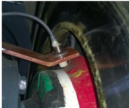
Fig. 4 Eddy current sensor for absolute angular positioning.
