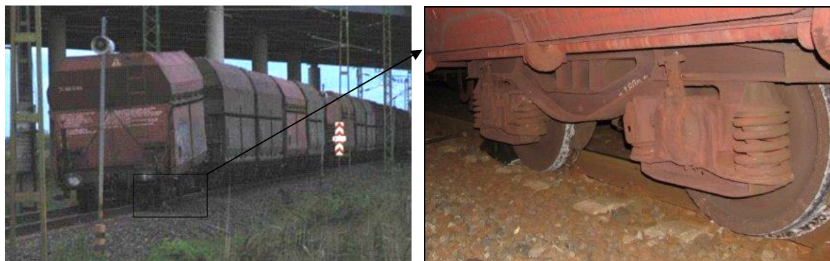
Fig. 1 Freight car after derailment
