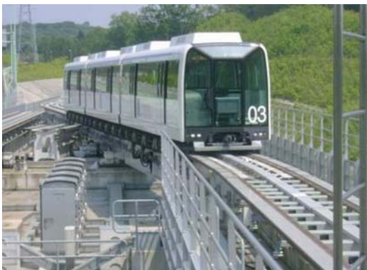
Fig. 1 Nagoya Japan the Lim driven levitated car
