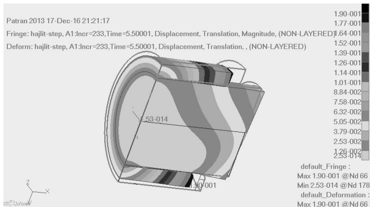
Fig. 5 Displacements at t=4.5 , maximal bending downwards
