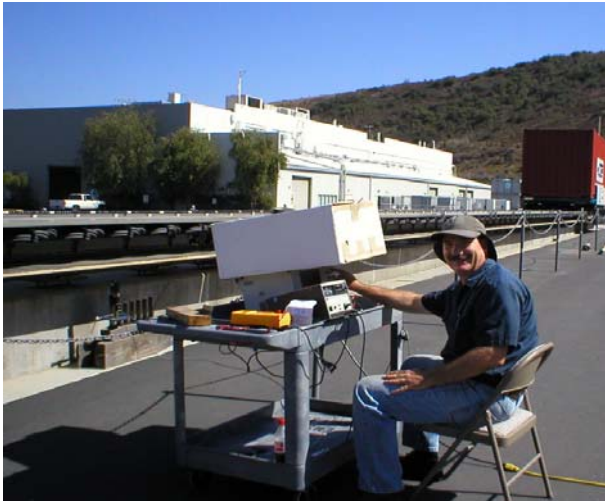
Fig. 11 Checking synchronization a typical LSM track
