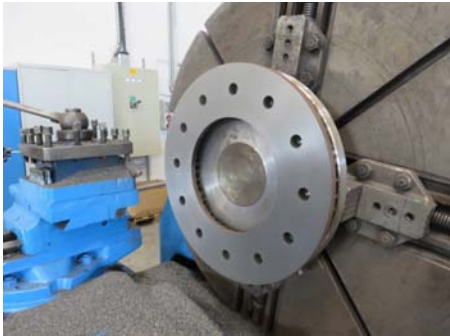
Fig.8 Wheel mounted brake disc under machining
