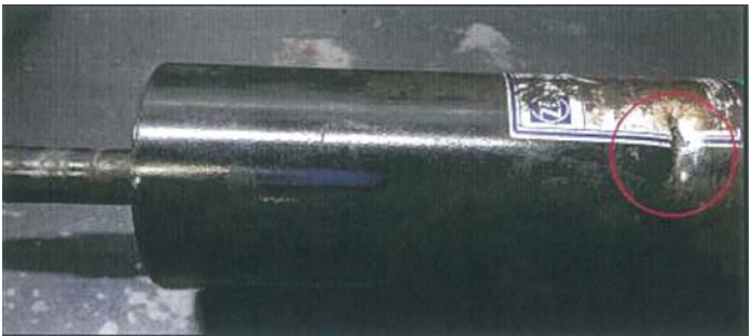
Fig. 3 Sample of a damper that has outlier damage
