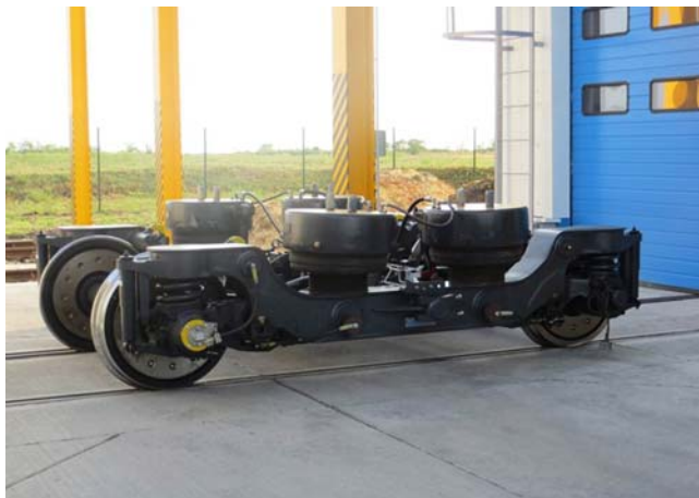
Fig. 11 Overhauled “Flirt” type Jacobs trailer bogie at BRCC
