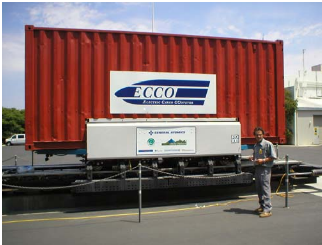
Fig. 5 LSM drive for container transportation
