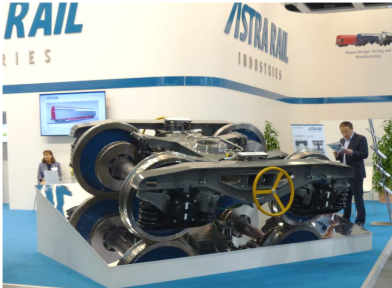
Fig.12 Prototype of Y25 disk brake bogie at InnoTrans Berlin exhibition
