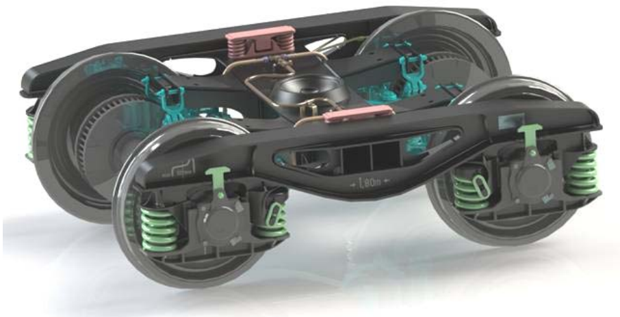
Fig. 2 CAD model of the complete Y25 disk brake bogie
